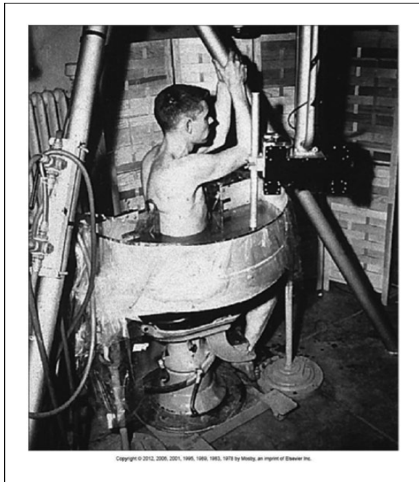
Figure 1. Photograph of the original Pan-scanner of Holmes et al 5 designed to allow ultrasonic visualization of the soft tissue structures of the human body. (Reproduced with permission; originally published in Hagen-Ansert SL: Foundations of Sonography. In Hagen-Ansert SL: Textbook of Diagnostic Sonography, 7th Ed, pgs. 2-20, Copyright Elsevier Mosby (2012).
